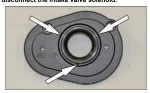
5. Install the provided venturi and the three throttle body mounting bolts into the back plate as shown. NOTE: The bolts pass through the back plate and venturi on the back side.
