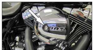
2. Remove the bolt which secures the bonnet to the filter assembly and then remove the bonnet from the vehicle.
