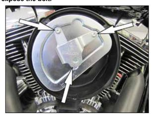
3. Remove the three bolts which secure the air filter to the filter base and then remove the air filter along with the crank case breather tube and bonnet bracket.
